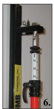
Adjusting Level Bubble. Most level bubbles have three screws to adjust the level bubble. You should only have to move one or two screws a slight amount to bring bubble back into center. If you have to move the screws a lot make sure screws are tightened evenly when bubble is level.
