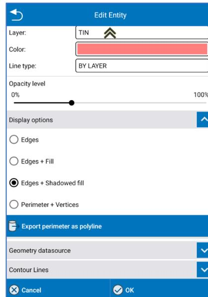
In this page at the top, you will see the section dedicated to name, code, layer, color and line type of the TIN. It is possible to select the opacity level between 0-100.
