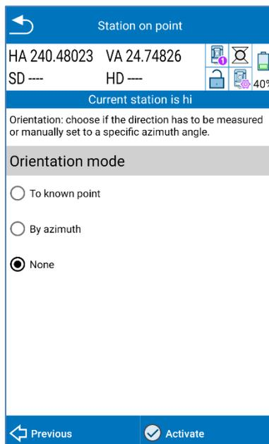
If you have *selected No Orientation*, you can click directly on *Activate* and you will complete the Station-by-Point procedure. Otherwise, in the other two cases, you have to click *Measure* and collect the measurement of the orientation point
