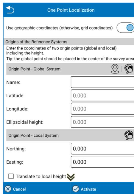
The function consists in assigning to a point, preferably central to the survey, the local coordinates that will represent the origin of the new local system.
