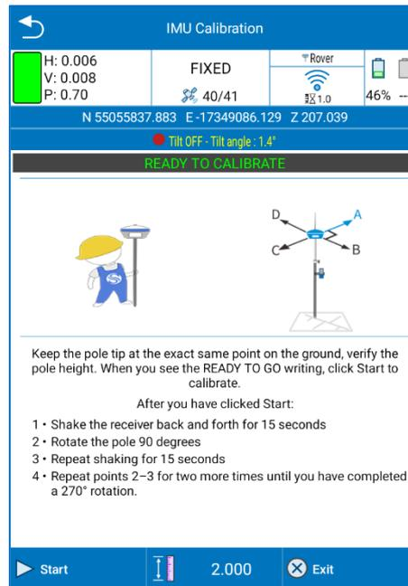
As shown in the following image, to calibrate the sensor correctly, you must first choose an arbitrary direction as a reference (direction A), then start moving the receiver back and forth along that direction until a message appears asking you to change direction.
