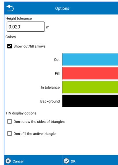
To access the *Options* menu, click on the icon at the top right. Here you can select the stakeout tolerance, display of cut/fill arrows, colour options and display options.
