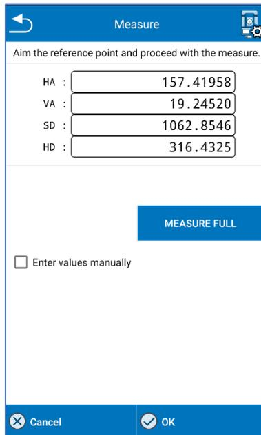
Where you can enter the total station control panel by clicking on
