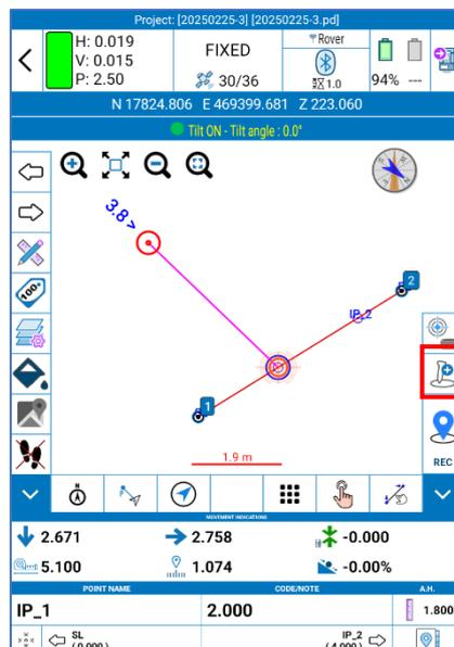
In the following example, the indications are for reach the point at chainage 0, with an offset distance of 100 meters on the right with respect to the line.
