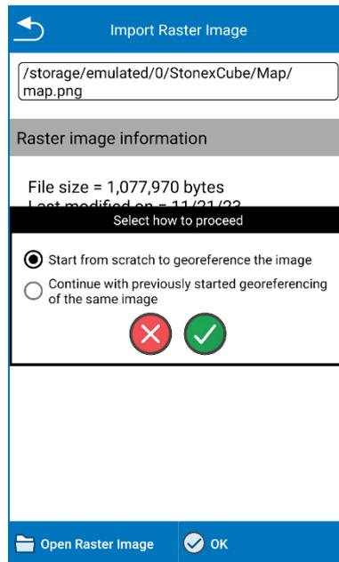
You need 4 points couples at least to perform the georeferencing. You need to associate the coordinates to 4 points not aligned at least in the raster image. You can take the coordinates from point library, from current GNSS position or from survey area.
