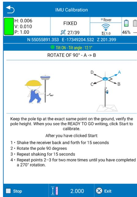
This operation must be repeated three times, then every 90 degrees up to a total of 270° clockwise.
