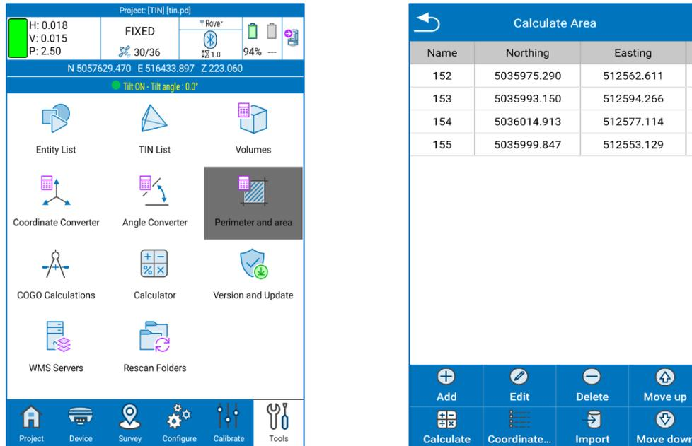
The screenshot shows the main application interface on the left and the 'Calculate Area' dialog on the right. The main interface displays various tools including Entity List, TIN List, Volumes, Coordinate Converter, Angle Converter, Perimeter and area (highlighted), COGO Calculations, Calculator, Version and Update, WMS Servers, and Rescan Folders. The 'Calculate Area' dialog contains a table with the following data:
