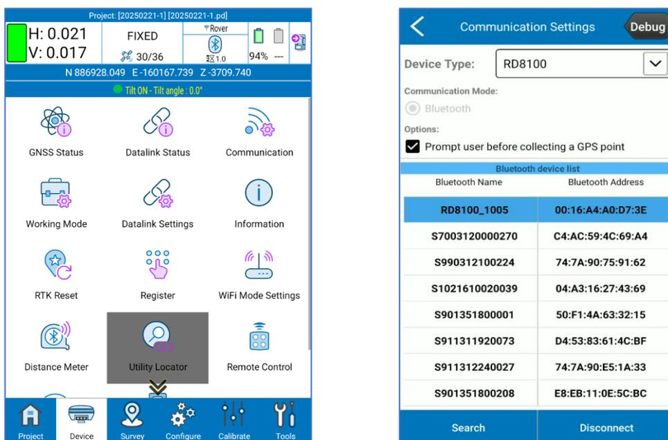
The first time you try to establish the connection, the pairing is required, and the password is 1234. Then, select the device and click **Connect**. See the detector user manual for more details on Bluetooth activation and locator settings.
