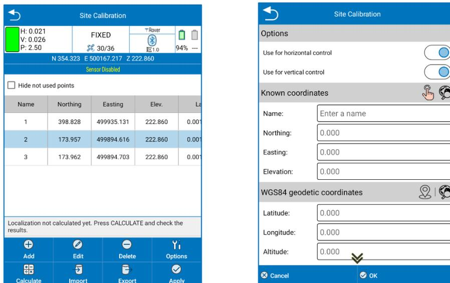
Added the point (or points) for localization, you can perform the conversion. There are three methods of converting coordinates: Inclined plane + Delta dimension (Roto-translation), 7 parameters + Inclined plane + Delta quota, 7 parameters, click the "Options" command in Figure, to access the reference screen in Figure.
