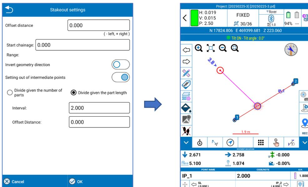
Click the icon in red in the following figure to stakeout specific points on the extensions of the line or on the shifted line.
