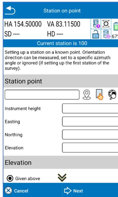
The elevation can also be inserted as a measure to a reference point. Define the reference point in the same way as it was done for the station point and insert the height of the target, then measure it and click *Next*.
