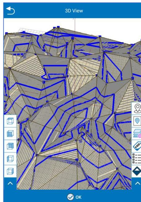
Contour lines can be optionally converted to real drawing entities and stored into a selectable CAD layer. If you select export as polylines in a layer, after defining the layer to export the polylines will be visible in the entity list.
