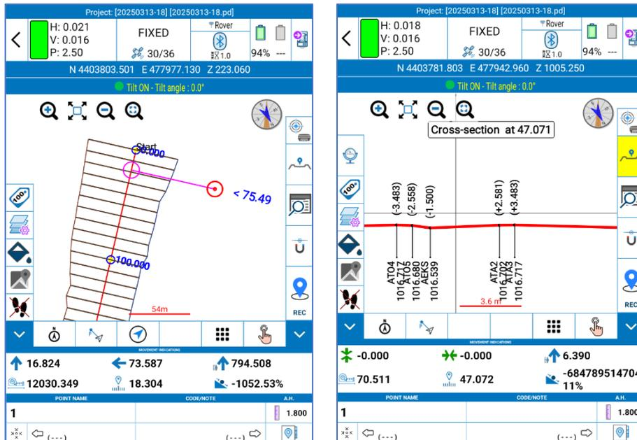
In the indication bar, in addition, there are the length and the chainage that is calculated from the projection of the current measure, and the following icons.
