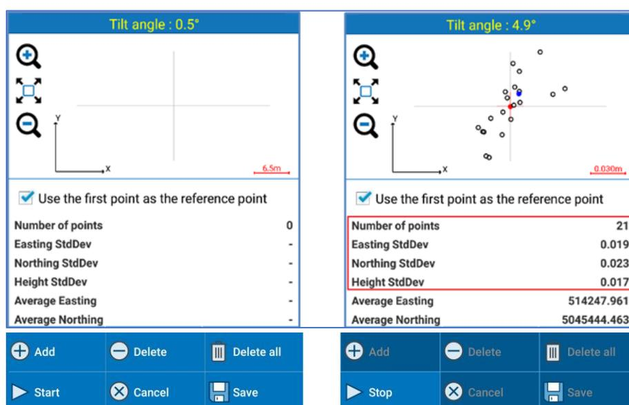
The user has control over the number of locations used in the calculation, and when he decides to end the control, he can press Stop to stop the automatic capture.
