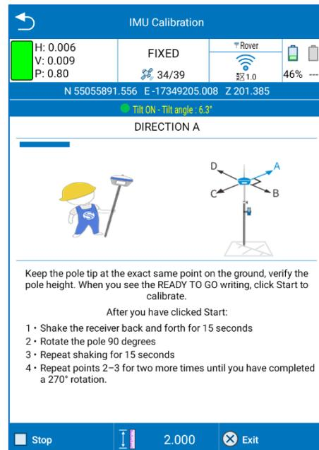
Then turn the receiver 90 degrees clockwise, reaching the direction  $A+90^\circ = B$ , and continue moving back and forth in the device.
