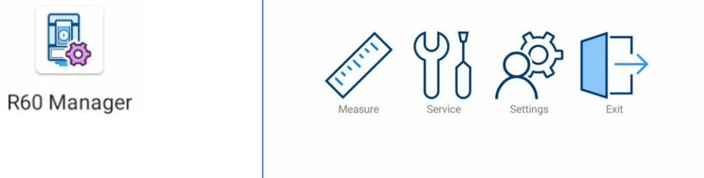
“R60 Manager” is organized in three menus: *Measure*, *Service* and *Settings*, as visible in the image above. In the screen upper bar, it’s possible to read the instrument battery level (top-left) and the total station FW version (top-right). Clicking on “Exit”, the user can close the application.
