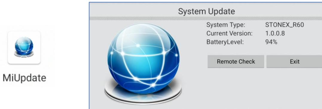
In this application, it is possible to read the current FW version (in the example above 1.0.0.8), verify the battery level (in the example above 94%) and check the presence of FW update.
