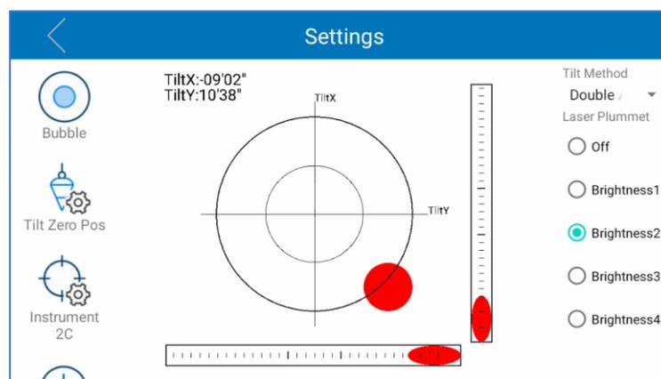
Use the tribrach leveling screws to level up the instrument, taking the electronic level on the screen as reference. Adjust the screws to make the bubble, visible on the screen, in the center of the electronic level, as visible in the image below.
