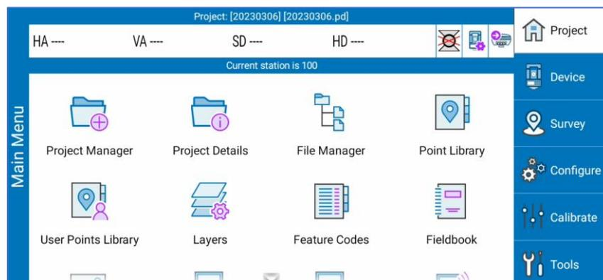
Click on "Device" -> "Total Station Communication" to check the status of the connection. Configure the instrument communication as in the photo below and click on "Connect" to activate the connection of the instrument with Cube-a.
