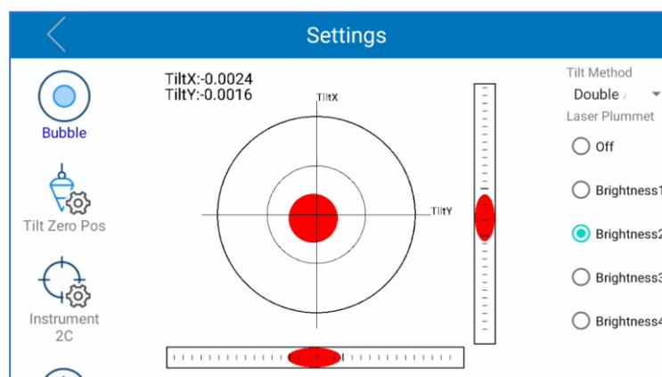
If plate level is not centered when leveling up with electronic bubble, probably it's necessary to calibrate it (see [5 Calibration](#)).
