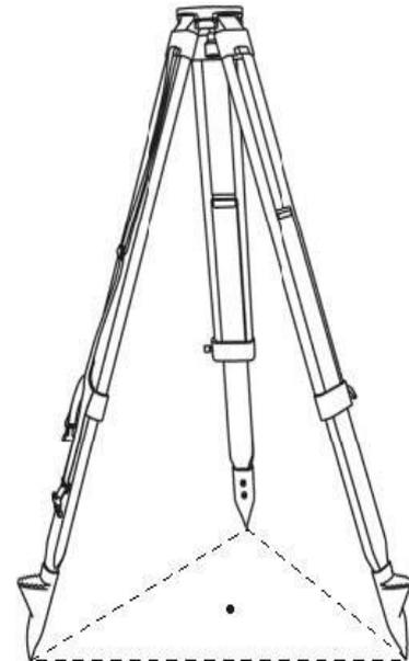
**Note 1.** The quality of the tripod setting up can affect the survey result. Remember to locate the tripod on a stable surface sticking the metal tips in the ground.
