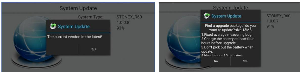
After instrument auto reboot, the following message appears. Click on YES to remove the old FW file from the instrument cache memory.
