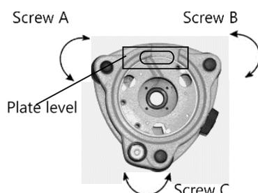
Turn the instrument till the plate level is parallel to a line shaped with screws A and B. Adjust the screws A and B to make the bubble in the center of the level.
