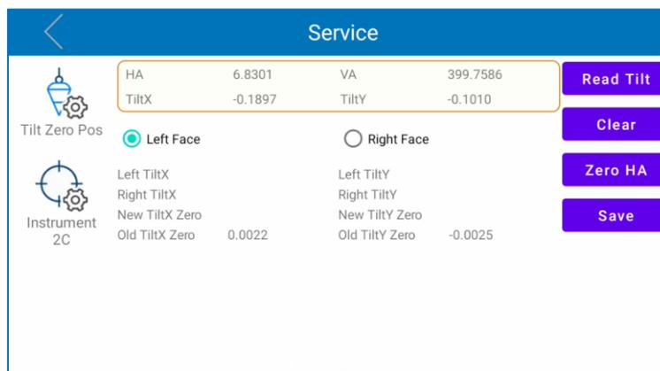
Two different calibrations can be performed in service menu: "Tilt Zero Pos" and "Instrument 2C".
