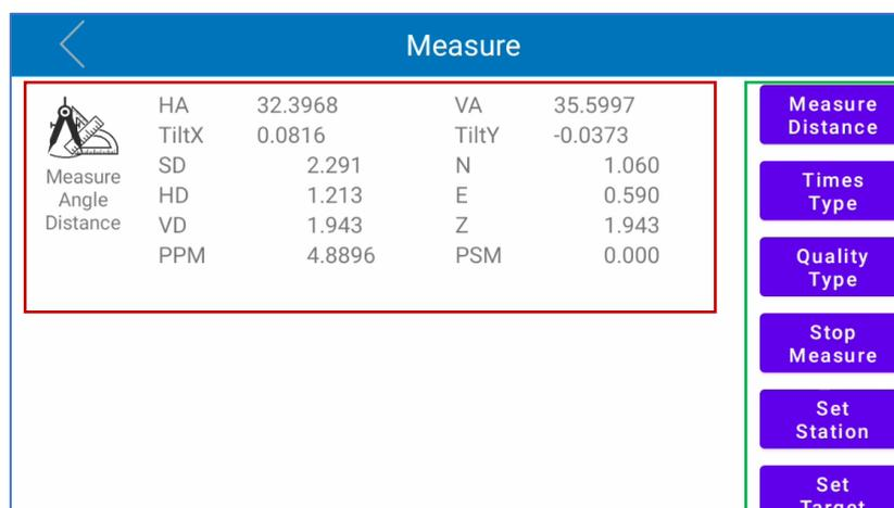
The central section (red squared in the photo above) contains all the information related to the measurements performed by the instrument. Below the list of the data included in this part:
