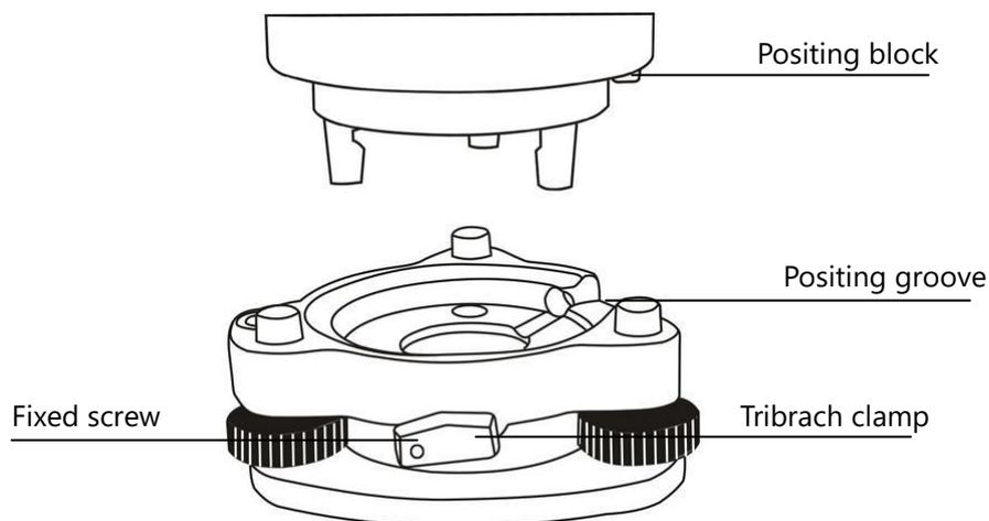
**Note.** If the instrument doesn't need assembly or disassembly from tribrach frequently, it is possible to fix the tribrach clamp by fixed screw to avoid the disassembly by accident. Screw out the fixed screw by driver to fix the clamp.
