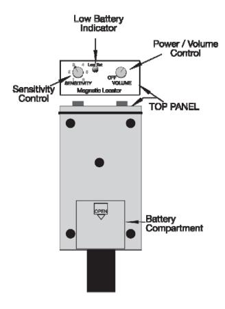
Figure 2: Instrument Controls
