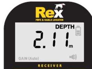
The display range for depth in feet and inches is 0" to 19' 11" and in meters is 0.00 m to 5.99 m.
