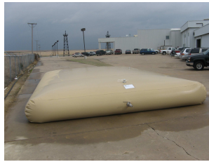
5,000 and 10,000 gal. Bladders Being Tested Before Shipping
