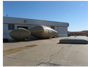
5,000 and 10,000 gal. Bladders Being Tested Before Shipping
