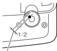
Adjust with the leveling foot screw
